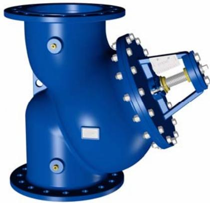
The Progressive Triple-Duty Valve combine pump discharge valve functioning as a shut-off, check valve and calibrated flow balancer. Available in sizes 2" through 18" with cast iron or ductile iron body.
