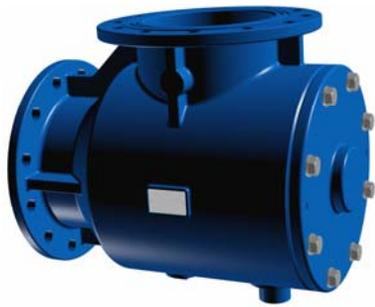
The Progressive Suction Diffuser is design to reduce space and installation costs by replacing a long radius elbow, strainer and extended entry pipe on the suction side of the pump. Flow stabilizing vanes reduce turbulence and resulting stress and vibration.
